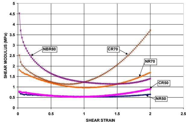
Figure 6: Variation of Shear Modulus with Shear Strain for NR, CR and NBR
