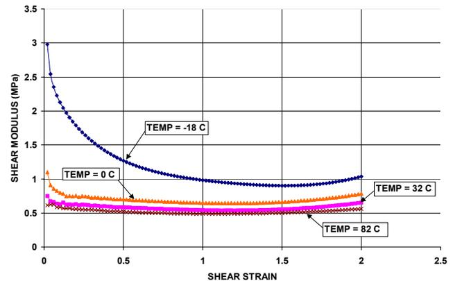
**Figure 14: Shear Modulus v/s Shear Strain for NR50 at Various Temperatures**
