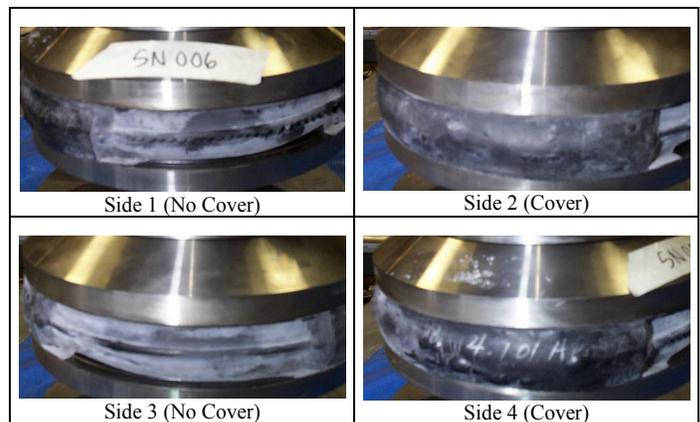
**Figure 12: Explosive Decompression Damage in 2.5 mm Specimen (Typ.) – 21 MPa Decompression Pressure**
