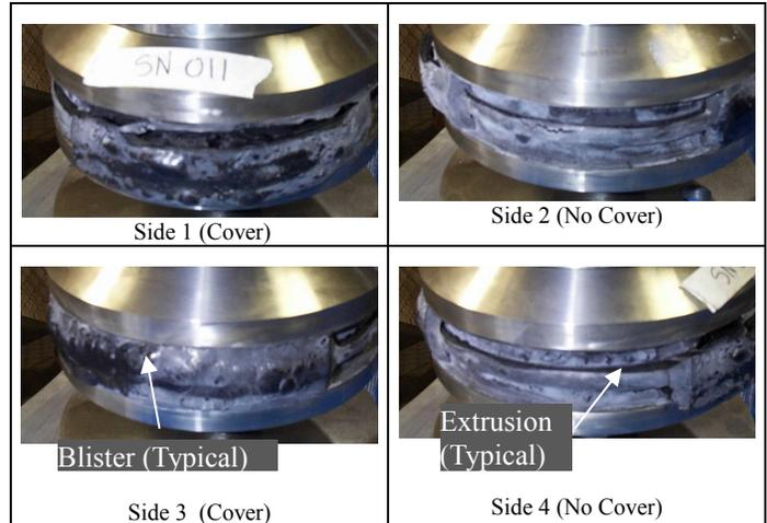
**Figure 10: Explosive Decompression Damage in 8 mm Specimen (Typ.) – 21 MPa Decompression Pressure**
