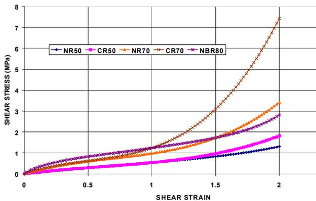
Figure 5: Stress-Strain Curve in Simple Shear for NR, CR and NBR
