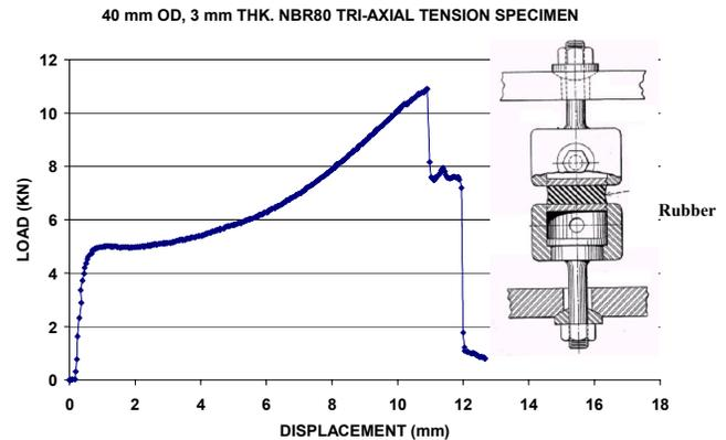
**Figure 9: Results of Tri-axial Tension Test (NBR80)**
