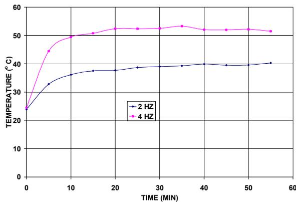
Figure 20: Change in Temperature of 25x25x6 mm Shear Specimen (NBR80)
