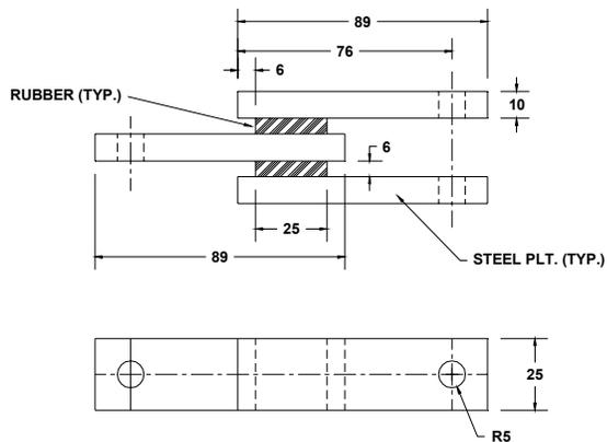
Figure 18: Configuration of Shear Specimen (mm)
