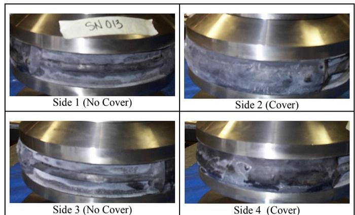
**Figure 11: Explosive Decompression Damage in 5 mm Specimen (Typ.) – 21 MPa Decompression Pressure**
