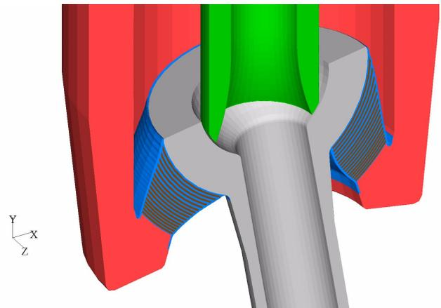
**Figure 4: Deformed Configuration of a Spherical Flex Element**
