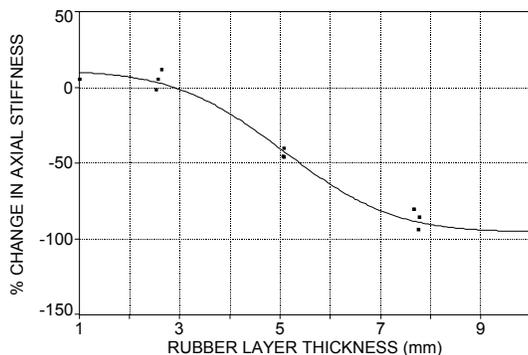
**Figure 13: Percent Change in Axial Stiffness due to EDD v/s Rubber Layer Thickness**
