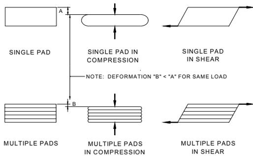
**Figure 2: Behavior of a Rubber Pad in Compression and Shear**
