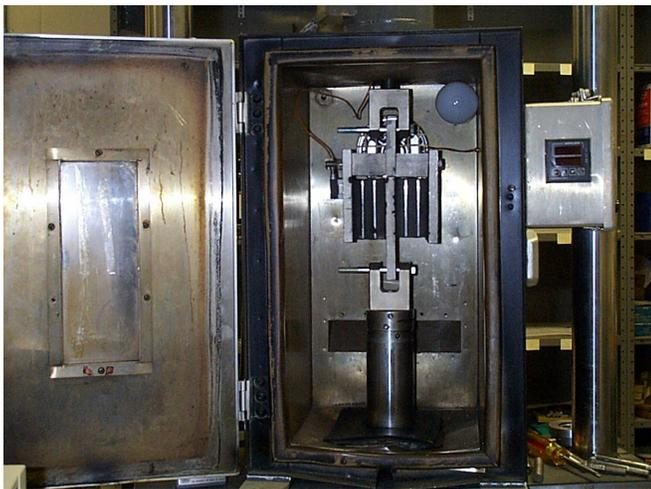
Figure 15: Test Setup for Accelerated Aging Tests in Shear Mode
