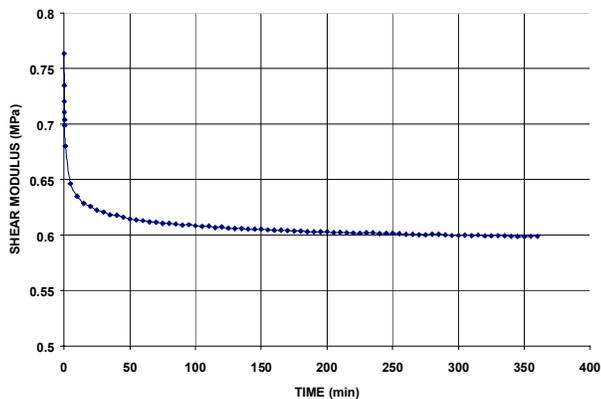
**Figure 8: Relaxation of Shear Modulus at 50% Shear Strain for CR50**
