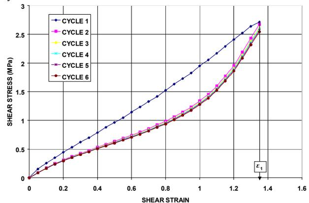
Figure 7: Stress Softening of CR70 in Shear
