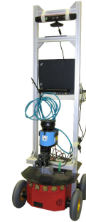
Fig. 8. The mobile platform we used for the experiments. Note that for this work we only exploit RGB-D data from a Microsoft Kinect sensor and do not make use of other sensors such as Laser Range Finder or sonars.
