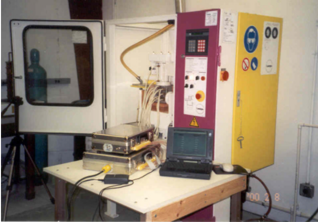
Figure 9. Experimental apparatus used to study dynamics of core shooting process.
