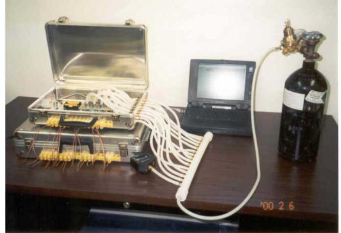
Figure 4. Experimental technique to study pressure losses in core box due to sand deposition in vent area during mold filling process.
