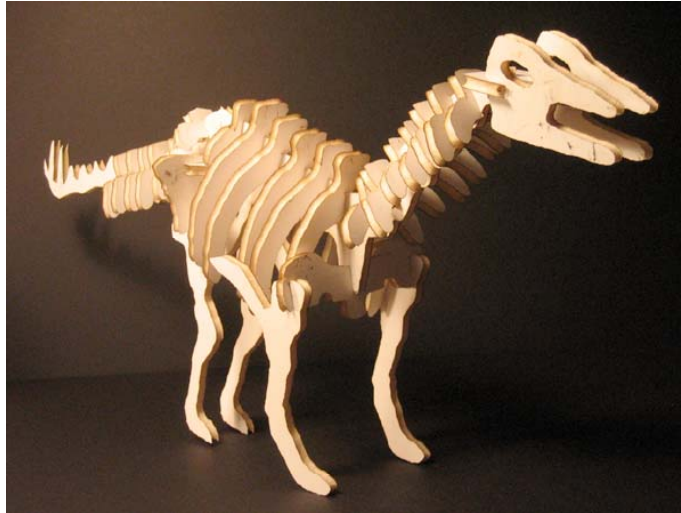
Figure 16. Made with the Designosaur: The authors created this dinosaur using the Designosaur system and a laser cutter. Compare with store-bought model, Figure 2.
