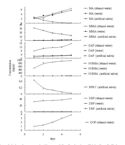
Figure 3. Rate of elution of monomers leaching out of Coe Comfort in artificial saliva, distilled water and binary mixture ethanol: water 40%:60% at every day monitoring at room temperature.
