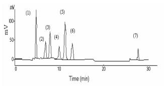
Figure 2. Typical chromatogram of the seven standard monomers.
