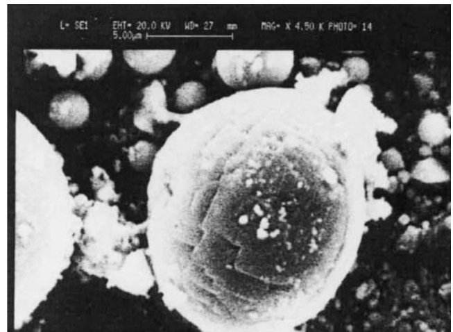
FIG. 6. SEM microstructure of plasma processed Al 2 O 3 /C powder in N 2 gas.
