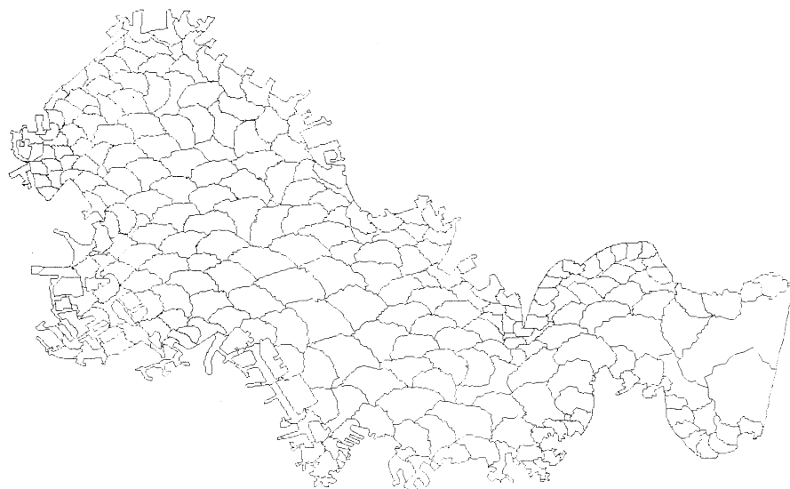
Fig. 6. Mesh partitioning for 256 processors
