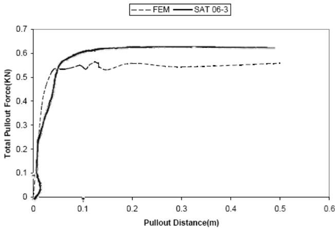
**Figure 6. Comparison of Pullout Force from FEM and Centrifuge Test**
