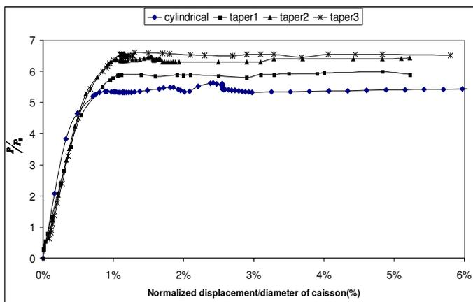
**Figure.7 Variation of Pullout Force versus displacement for caissons with different taper angles**
