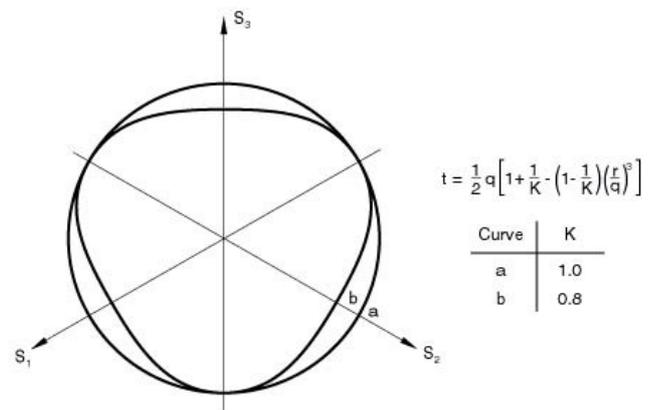
Figure 4. Modified Cam-Clay yield surfaces section in  $\beta$  plane
