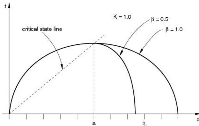
Figure 3. Modified Cam-Clay yield surfaces in p-t plane
