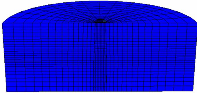
Figure 2. Typical finite element mesh for  $l/D = 3.5$
