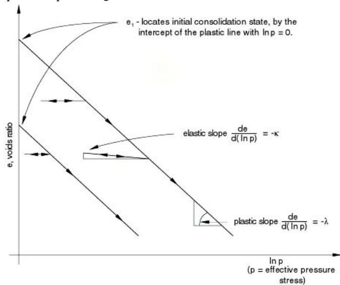
**Figure 5. pore compression behavior for clay model**
