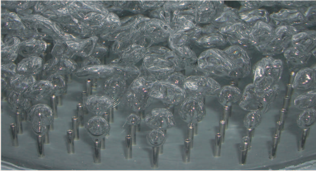
Figure 1: A photo of a needle sparger used in a slurry bubble column with one-third of the needles in operation. By using long needles instead of holes, a much higher pressure drop is achieved, which leads to a much more uniform bubble size and consequently a lowered E_L . [31].
