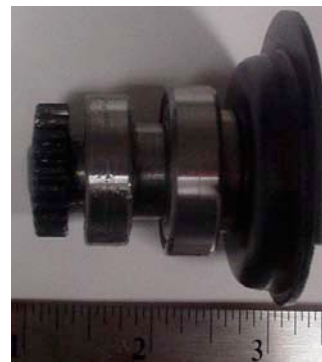
Figure 9: Drive Train Assembly of Delta Sander
