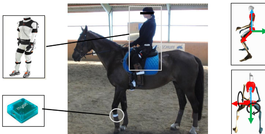
Fig. 1. Experimental setup: rider (MVN suit) and horse (acceleration sensor on the cannon bone) with the applied measurement systems: rotation axes of the riders' segments are shown as arrows: red arrows indicating Roll angles and green arrows indicating Pitch angles.
