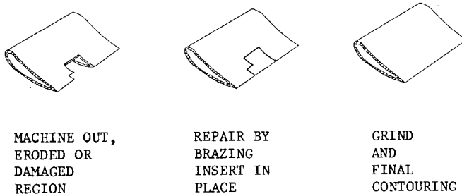
Figure 25: Schematic representation of a brazed replacement insert method for repairing cracks on nozzle aerofoils
