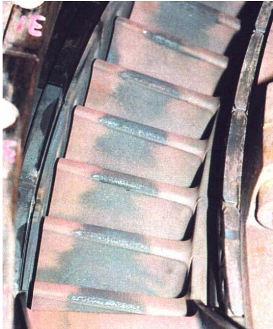
Figure 10 – Case history 3: cyclic oxidation damage on mounted first stage blades, leading edge side.
