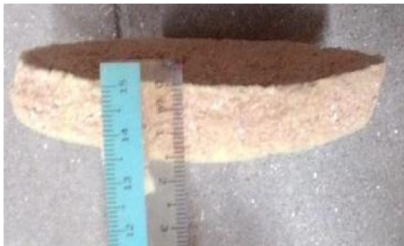
Fig 15: Polyurethane layer after test becomes thinner
