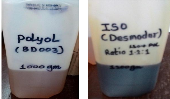
Fig 6: Mix ratio of polyurethane compounds
