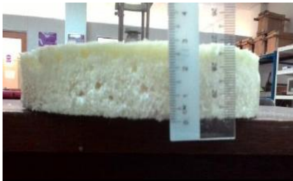
Fig 14: Polyurethane layer before test
