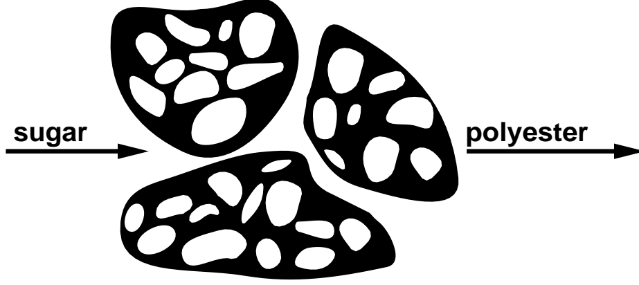
Figure 2: Biopolymerization: bacteria eat sugar and produce polyester. White areas: polyester granules within bacteria cells.
