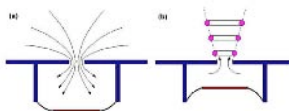
Figure 1. A schematic of synthetic jet operation
