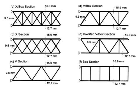
**FIGURE 51.4** Shapes considered for design of a truss-type composite bridge deck. (a) X/box section; (b) X section; (c) V section; (d) V/box section; (e) inverted V/box section; (f) box section.
