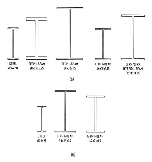
**FIGURE 51.1** Comparison of different beams for a two-lane 16.80-m-span bridge, with a total of five beams spaced at 2.30 m, and a 180-mm-thick concrete slab. (a) Noncomposite action between beams and slab; (b) composite action between beams and slabs.
