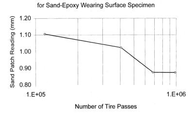
FIGURE 51.6 Sand patch test readings for sand-epoxy wearing surface specimen.
