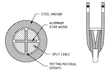
FIGURE 51.2 Potted end anchorage assembly for composite cables; cross sectional view (left) and longitudinal view (right)
