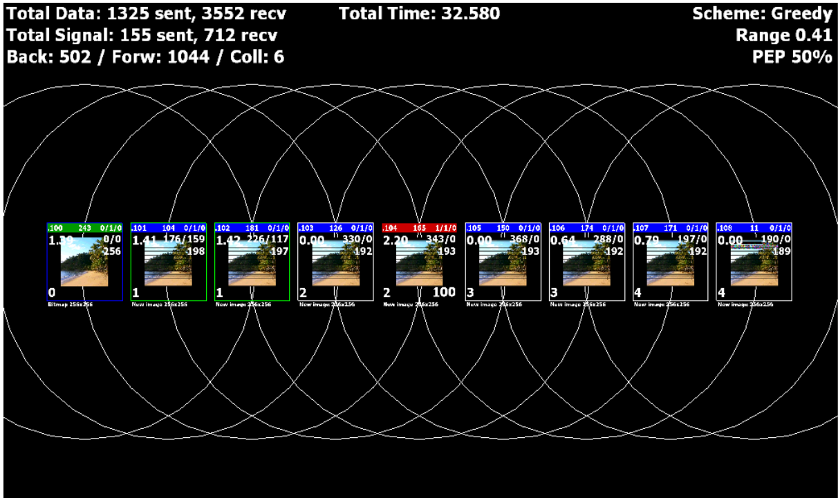
Fig. 1. Screenshot of the simulator showing 9 nodes. The leftmost node was chosen as the initial source. Nodes in green are complete. Nodes in blue are in progress. Nodes in red are transmitting at the moment.
