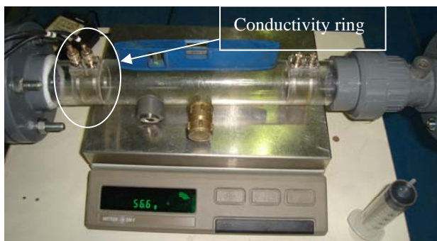
FIGURE 9, CONDUCTIVITY RING STATIC CALIBRATION
