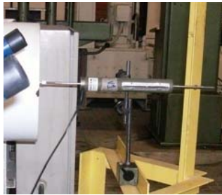
Figure 8 – Detail of the displacement transducer 1.
