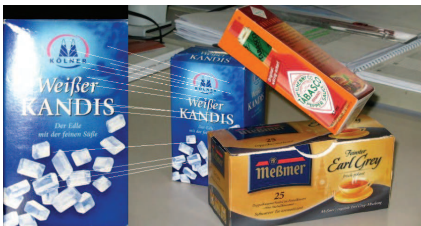
Fig. 1. SIFT feature matches applied to a self recorded scene. The blue sugar box on the left side of the image was found in the right complex scene. The SIFT matching software yielded 16 matches (shown as white lines). Note that only 3 matches would have sufficed to correctly identify an object. Also note the partial occlusion and difficult lighting conditions under which the images were taken. The digital camera used to record both images was a Canon Powershot A75 with 3.2 megapixels. The camera was set to automatic mode. The images also underwent a lossy JPEG compression.
