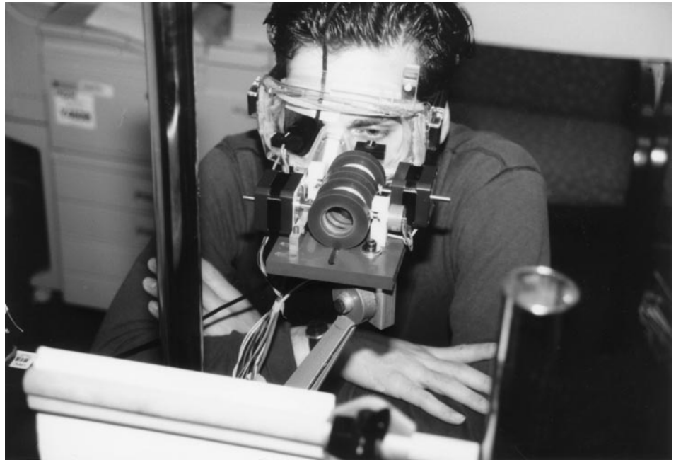
FIGURE 1. One of the authors models the prototype device. He wears a pair of goggles that holds the infrared eye movement probe and looks through the table-mounted, motor-driven prism assembly. The edge of the support used to hold acuity test cards is visible in the foreground.
