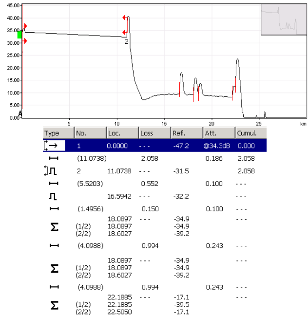
Figure 5. The network testing results for line 1 for the OTDR trace of downwardly testing in the proposed system architecture and the event table for OTDR trace
