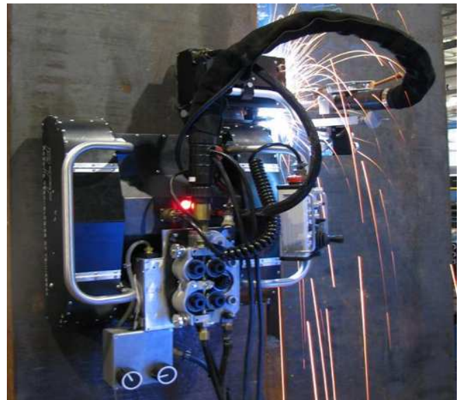
FIGURE 2: MRWS CONDUCTING A WELD
