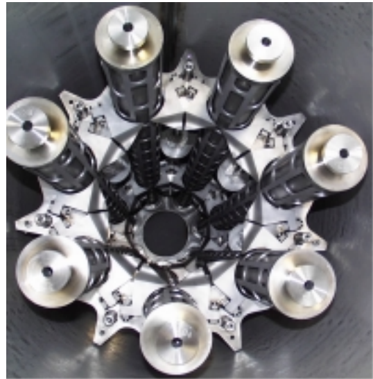
Figure 3 - Canister inside view showing rack, cans and magazines before pouring glass
