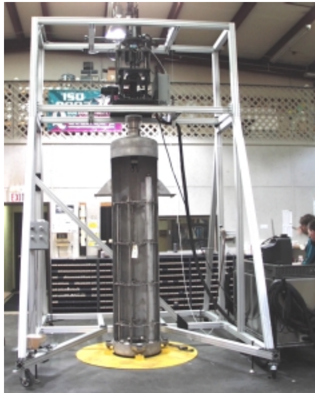
Figure 6 - Canister Loading Robot Mockup
