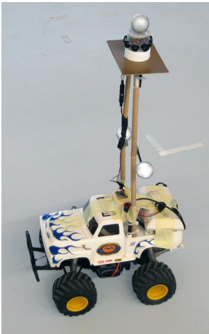
Fig. 2. The ultrasound beacon mounted onto the top of a R/C model car. For ground truth information reflective MoCap markers are attached to the car and the beacon and allow for precise high-speed tracking of the position of the beacon.
