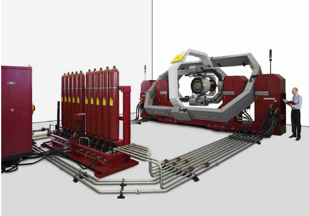
Fig. 3. The series HD7736 FMS including the two axis HD7727-T TMS. In addition to the parameter shown in Table 1 the system required a large UUT of 1m length, 176kg mass and up to 0.5m diameter. The roll/yaw and pitch axis are continuous/ \pm 60^\circ and +100/-140 respectively. Note the accumulators and the piping to the simulator which require considerable installation time.
