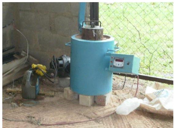
Figure 4: The salt bath furnace after Installation
