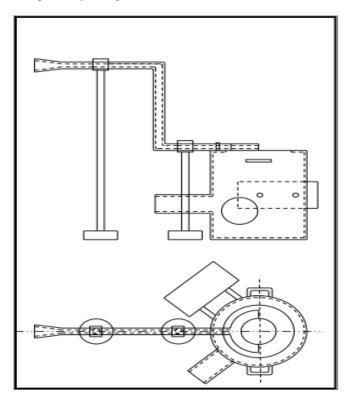
Figure 1: Orthographic view of the Salt Bath Furnace
