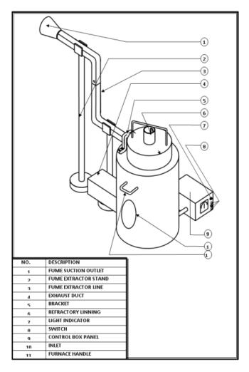
Figure 2: Isometric View of the Salt Bath Furnace
