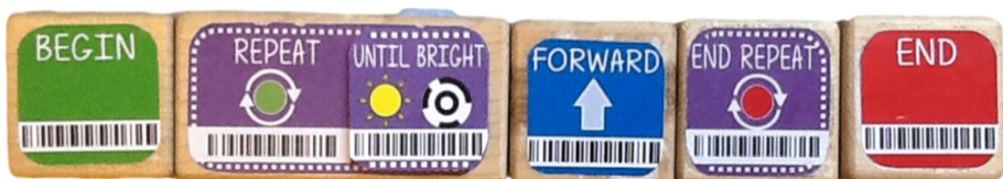
Fig. 8 Programming blocks for Light Sensor Program. Using this type of program, children programmed their robots to continue forward along the map until a flashlight shines into the light sensor. Once the light is detected, the robot stops moving
