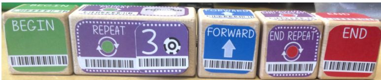
Fig. 6 Repeat Loops Program. This figure illustrates a CHERP program that would tell the KIWI robot to move forward three times and then stop
