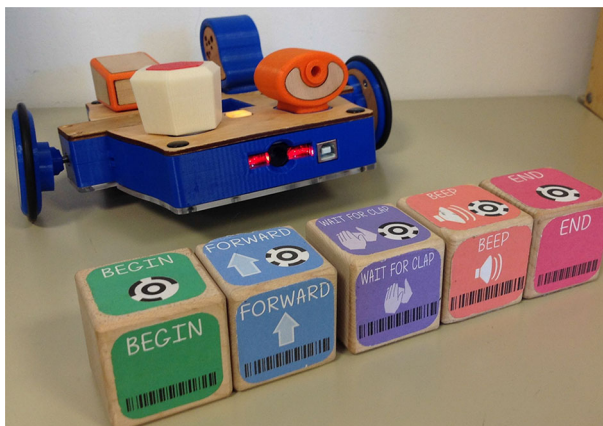
Fig. 2 KIWI robot prototype and CHERP programming blocks
