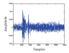
Fig. 19. Reflected signal by. pedestrian placed at 2 m.
