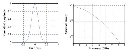
Fig. 1. Gaussian pulse time and spectral representations.
