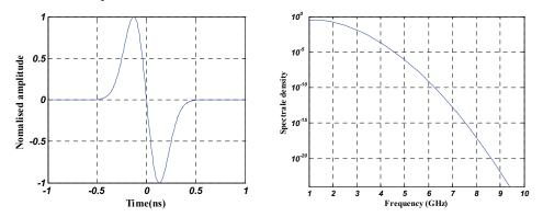
Fig. 2. Monocycle pulse time and frequency representations.
