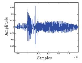
Fig. 20. Correlation signal using a pedestrian at 2 m far from radar.
