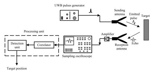
Fig. 3. The radar based on UWB pulses.
