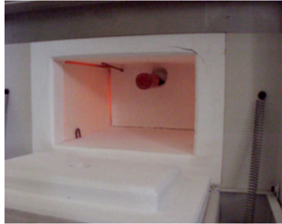
Figure 3: Sensor packaging in a laboratory furnace and simultaneously loaded with pressure up to 300bar.
