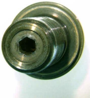
Figure 2: Test packaging after about one week of leakage test simultaneously stressed from RT to 600^\circ\text{C} .
