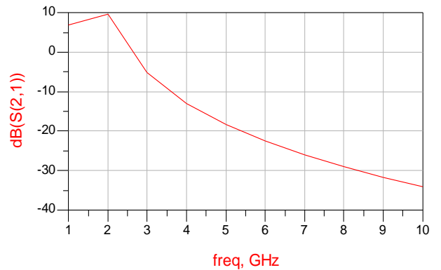
Fig 11. dB(S21) Low Noise Amplifier With Component Element ADS
