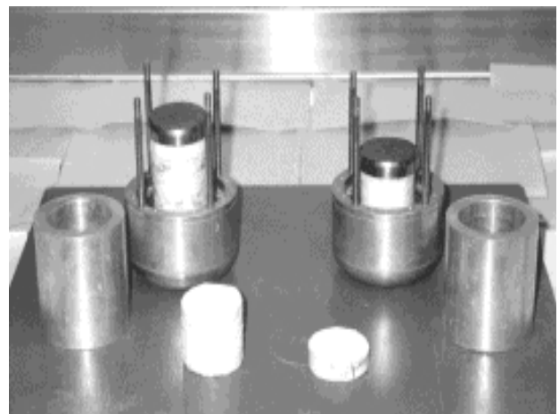
Figure 4. Saturated soil specimens on top of the saturated ceramic cylinders in the drainage plate.
