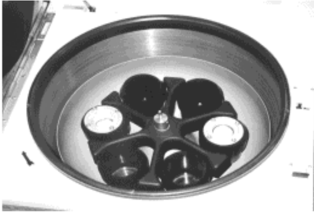
Figure 5. Soil specimen holders in the centrifuge buckets ready for centrifugation.
