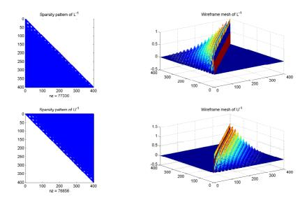
Figure 2: The 2D driven cavity problem: sparsity pattern (on the left) and wireframe mesh (on the right) of the inverses of the L and U factors obtained from the ILU factorization of the Jacobian at the starting point (n = 400, Re = 50).
