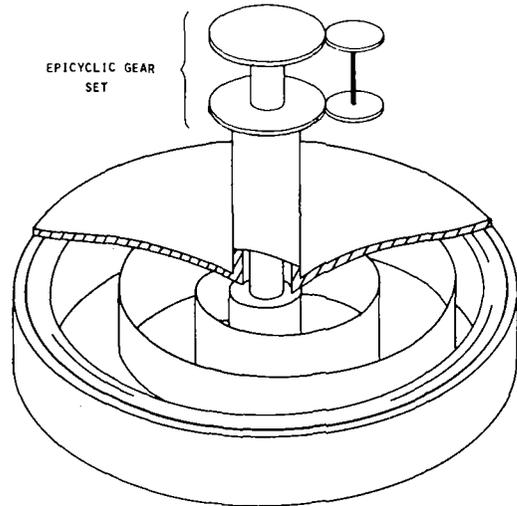
Fig. 7 Fixed ratio power recirculation variable inertia flywheel
