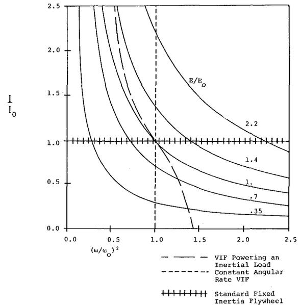
Fig. 3 Variable inertia flywheel isoenergy plot
