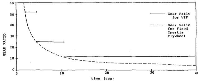
Fig. 6 Gear ratio of transmission for the variable inertia flywheel powering an accelerating automobile
