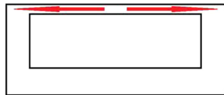
Fig. 12 Heat transport situation in downfacing structures
