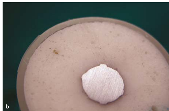
■ Fig. 5.5. a Implant and cement in syringe. b Shrinkage gap between cement and syringe; porosity in cement forced away from implant towards syringe
