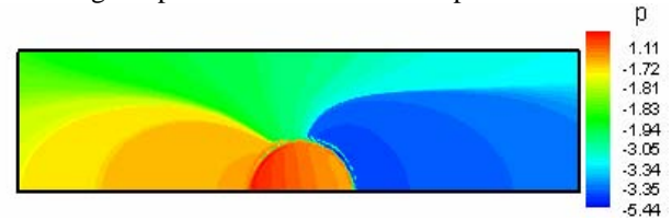
Fig. 2: Pressure contours across a droplet in a channel flow.
