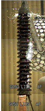
Figure 5 – Flashover test, Lower A1 section, V = 500 \text{ kV}_{\text{rms}} , 5 mm/min
