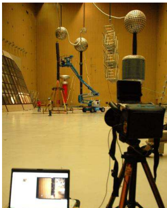
Figure 3 – Test layout, including the position of the daylight UV camera
