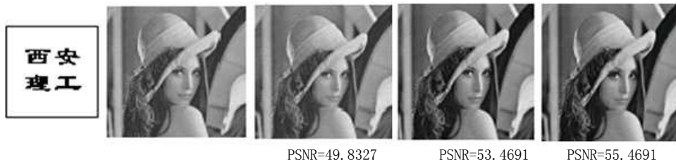
(a) Watermark logo (b) Original Image (c) DWT-Only (d) DWT-DCT-Only (e) The proposed method Fig. 4 Comparison between original images and their corresponding watermarked images
