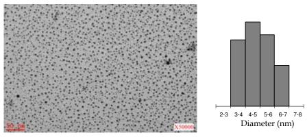
Fig. 3. TEM image of silver nanoparticles embedded in a polyacrylate matrix, with the corresponding size distribution
