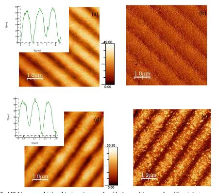
Fig. 5. AFM images obtained in tapping mode of holographic records without Ag<sup>+</sup>, (topography (a), phase (b), cross-section (inset)); and with Ag<sup>+</sup>, (topography (d), phase (e), cross-section (inset)) (Reprinted with permission from ref Balan et al., 2009. Copyright 2009 ACS)
