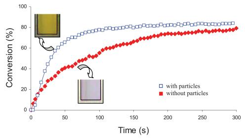
Fig. 1. Real-time FTIR kinetic conversion curves for visible curing at 532 nm of resins with and without particles (Insets: View of 30  $\mu$ m thick samples with and without nanoparticles after curing)
