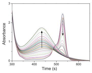
Fig. 2. Time evolution of the absorption spectrum of the resin during photopolymerization  $EO^2$ / MDEA / AgNO<sub>3</sub>, (0.1 / 3 /1 wt %)
