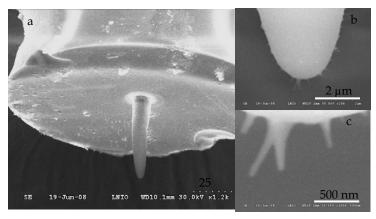
Fig. 8. Silver/polymer composite tip integrated at the end of an optical fiber and zooms of the extremity of the tip showing silver nanowires. Light Power =  $2 \mu W$ , exposure time = 5 s (Jradi et al., 2010. Copyright 2010 Nanotechnology)
