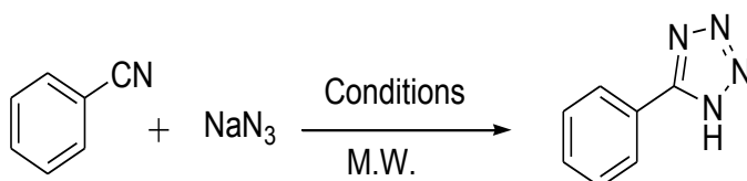
Scheme 1. Synthesis of 5-phenyltetrazole under microwave irradiation.
