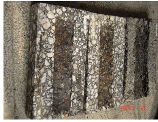
(b) Specimen after Rutting Test.
