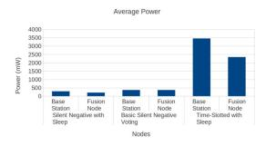
Figure 14: Average power consumption for TelosB
