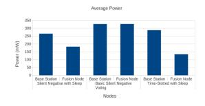
Figure 4: Average power consumption for TelosB
