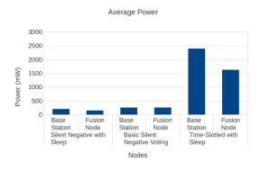
Figure 12: Average power consumption for Mica2
