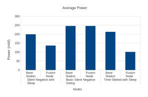
Figure 1: Average power consumption for TI CC1100
