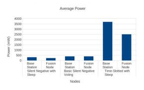
Figure 13: Average power consumption for MicaZ
