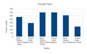
Figure 3: Average power consumption for MicaZ
