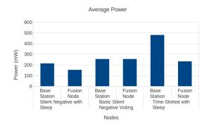
Figure 6: Average power consumption for TI CC1100
