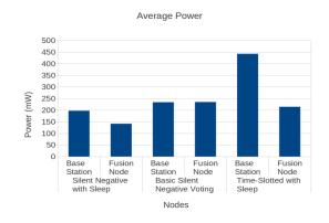
Figure 7: Average power consumption for Mica2
