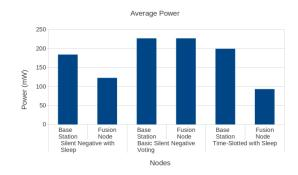
Figure 2: Average power consumption for Mica2
