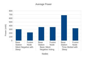
Figure 9: Average power consumption for TelosB
