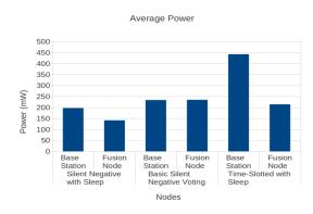
Figure 8: Average power consumption for MicaZ
