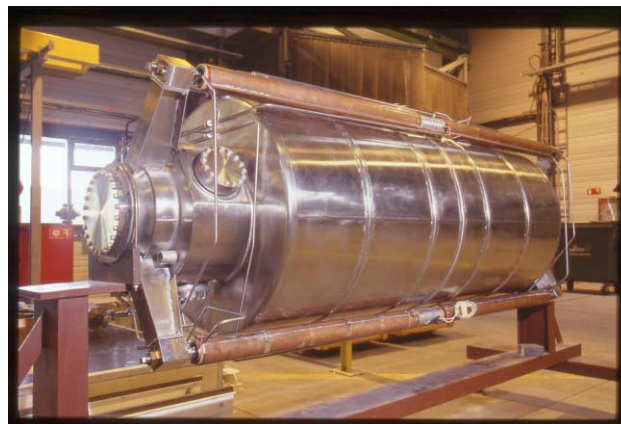
Figure 1, Five cell \beta=0.85 Trasco Cavity housed in the helium tank
