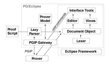
Fig. 7. PG/ECLIPSE system architecture.
