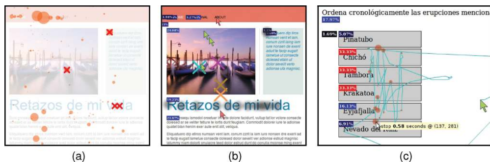
Fig. 1. Combining visualization possibilities. (a) Displaying hesitations (circles) and clicks (small crosses). (b) Displaying entry/exit coordinates (cursor bitmaps), motion centroids (crosses), highlighting activity (shaded fog), and interacted DOM elements (numbered rectangles). (c) Analyzing a decision process; the user rearranged items in a list. Small circles represent cursor dwell times. Hovered DOM elements are labeled based on frequency (percentage of browsing time), including a blue color gradient (100% blue: most hovered items). The same scheme is used to analyze clicked items but using red color.
