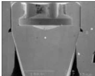
Fig 7a (Left) SEM of hand-tightened synOcta implant with synOcta 5.5-mm solid abutment ( \times 37 ) showing the abutment screw (s), abutment (a), and bearing ring (b).
