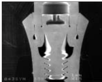
Fig 6a SEM of synOcta implant with synOcta 5.5-mm solid abutment ( \times 15 ) showing the 2-piece abutment connection.
