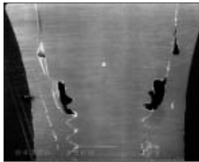
Fig 5a (Left) SEM of synOcta implant with 5.5-mm solid abutment ( \times 23 ) showing abutment (a) and implant (i).
