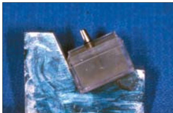
Fig 1b Specimen supported in stainless steel block with an incline of 30 degrees.
