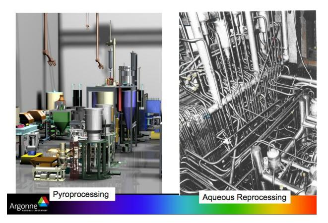
The relative simplicity and small size of pyroprocessing systems vs. aqueous systems is graphically illustrated above. The entire recycling system for an IFR power plant could be contained in a hot cell about the size of a large garage, while aqueous reprocessing systems are extensive, complex, energy intensive and costly industrial enterprises.
