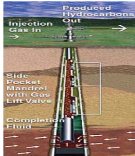
Fig. 2: Schematic of a gas lift well
